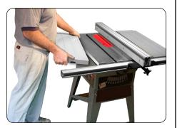
Remove the factory left extension wing. If the bolts for the existing table saw wing are grade 5 and are 1 1/2" long save them for reuse in mounting the Cast Iron Router Wing.
