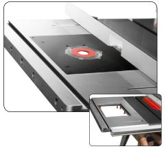
Install router insert plate into the Cast Iron Router Wing. Adjust the leveling screws until the plate is flush with Cast Iron Router Wing. You are ready to mount your router.
